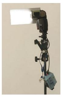
To make a useful-sized GoBo, Cut a piece of still cardboard to make a rectangle about 4x8 inches. Cover it with gaffer's tape and stick some Velcro (the "hooks" side) at one end and at about a third of the way from the other end. This will allow you to attach it to the side of your flash either way so that you can choose how far it sticks out.
