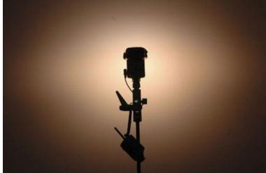
This is a flash fired against the wall (4 feet away) at the "85mm" zoom setting. Note the pattern of the light.
