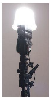
And if you a bit of a DIY-type, keep an eye out for a piece of tupperware container that will do the same thing for your strobe. You can either find a bottom that will scrunch onto your flash, or cut an "X" in the lid about the same size as the cross section of your flash head and just slide the closed container on. Just be mindful (as in test) to make sure the tupperware is not giving you an unwanted color cast.
