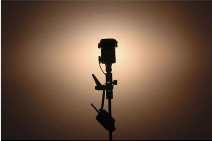
This is a flash fired against the wall (4 feet away) at the "85mm" zoom setting. Note the pattern of the light.
