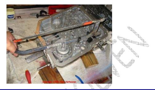
Notice the two valve body screws 70 to hold down the hacksaw.
