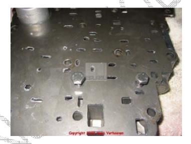
Use a couple or all the twelve valve body screws 70 to get proper alignment of the plate and gaskets. Use 13 Nm of torque (9.58 Ft lb or 115 in lb) to tighten.
