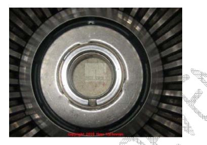
As with the 3rd clutch assemble steel plates 626 and lined plates 627 into a stack.
