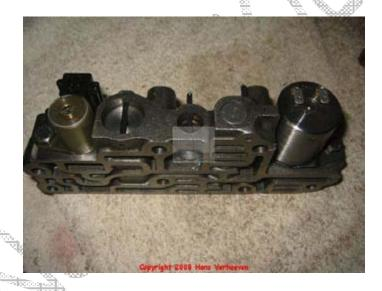
Before sticking the adapter case valve body 401 the wiring harness has to go in place. Route it through the channel in the adapter case before you put the completely assembled adapter case valve body 401 on the adapter case. Stick in the seven screws 70 and hand tighten them.
