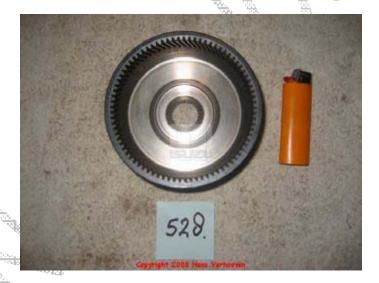
Note that the overdrive internal gear 528 only turns counter clockwise and blocks in the opposite direction. This is what it is designed to do. I am not getting to technical here as we're only rebuilding a trans ©.
