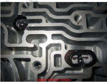
Next stick the transfer gasket main case 88 on with petroleum jelly to hold it in place.
