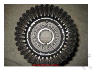
Place the 22 piston springs 611 on the  $2^{nd}$  clutch piston 622.
