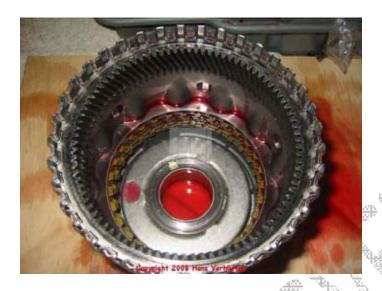
And finally the other retaining ring 629 to hold the ring gear 630 in place.
