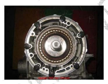
First find out how the steel plates fit in to the adapter case.
