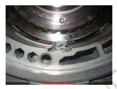
Start putting the reverse clutch plates 615 and reverse lined plates 616 together.
