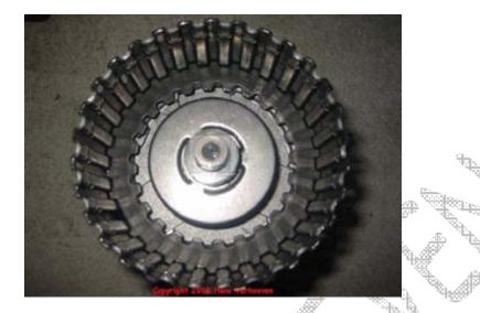
Install retaining ring 640 on inner piston while compressing spring seat 639 down. Make absolutely sure the retaining ring is falling within the cavity of the spring seat.
