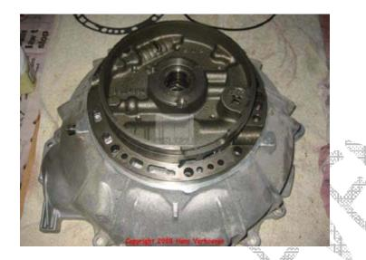
Turn the converter housing 6 on its side and install the five screws holding the oil pump assembly 10. Go hand tight (loose) for now. DO NOT install the converter housing ring seal 3 yet.
