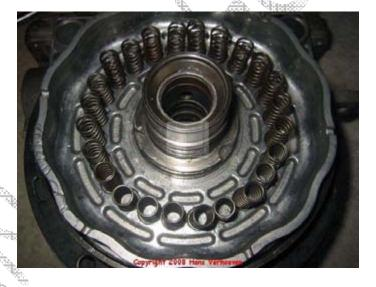
Place all 24 springs 611 into the slots on the inside the reverse piston 610. Put the spring seat 612 on top of them.
