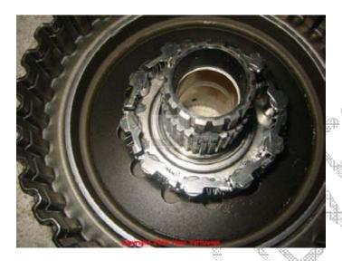
Gently put the overdrive roller clutch cam 517 in the roller assembly 516.
