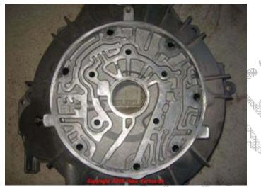
Place the oil pump body wear plate 9. You can not install this one wrong. The holes for the screws won't match up if you tried.
