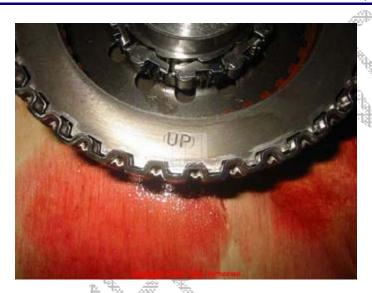
Install snap ring 524 onto the overrun housing.
