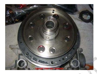
Use the eight screws 31 to fix the center support 30 on the adapter case 20.
