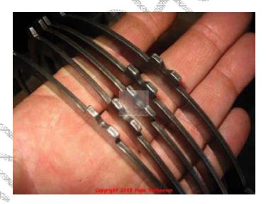
Take extra caution here. If you take a good look at them you will see that they have a groove on one of the notches. They must be installed with the groove at the lowest point of the main case. I believe this is to ensure proper oil flow through the oil channel in the bottom of the main case 36. See the next picture
