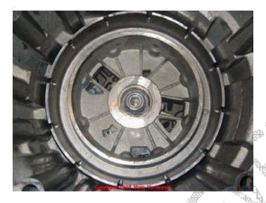
Place the retainer and spring assembly 531 with the retainer facing upwards inside the 4th clutch piston and install the snap ring 530. Ensure it is completely fitted into the groove.
